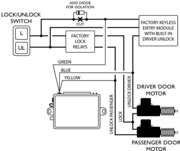
The door lock switches output a positive trigger, and the door lock relays are usually separate from the keyless entry module. In this system the keyless entry module features a built-in relay to unlock only the driver door.
