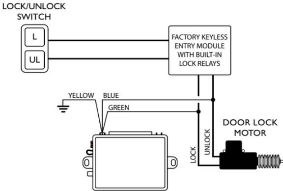
When connected as shown below, the system will arm or disarm with the keyless entry transmitters and with the door lock switches. If the vehicle is equipped with two-step unlocking, it is strongly advised to follow the directions for *Universal Two-Step* instead.
